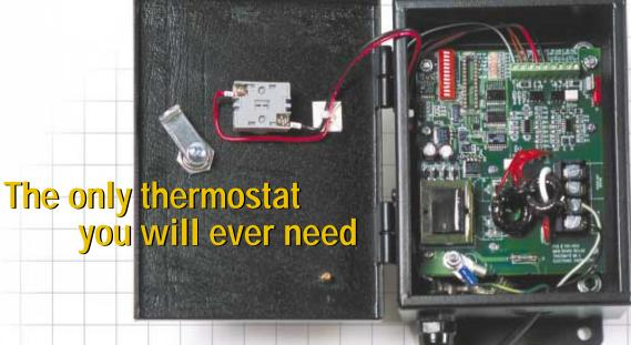
The new TRACEMATE<sup>™</sup> from Nextron Corporation meets all your heat tracing control and monitoring needs in one convenient, compact, competitively priced package.
