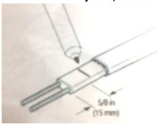
6. Trim the bus wires to a length of ½ inch (13mm). Connect the heating cable bus wires to the leads on the lighted assembly by way of supplied crimp connectors.
