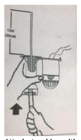
3. Attach stanchion with pipe clamp. Do not tighten pipe clamp over cable.
