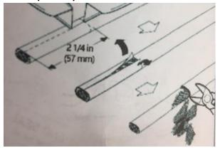
5. Remove the inner jacket, and heating core exposing bus wires.
