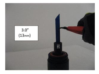
**10.** Trim / remove the outer jacket and ground braid 0.5" (13 mm) from the end of the cable.
