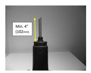
**6.** Tighten the connector until it bottoms out.
