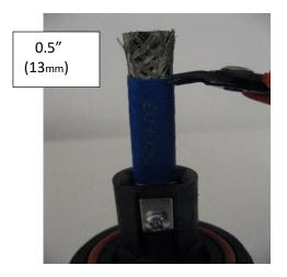
**11.** Slide the Silicon Boot over the end of the cable. Ensure the lower O-ring is in place.
