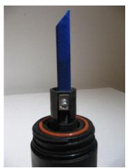
**8.** Tighten the Strain Relief Screw to secure the cable.
