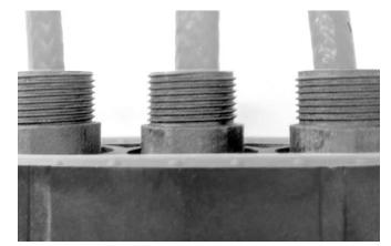
Cut outer jacket flush with connector and
