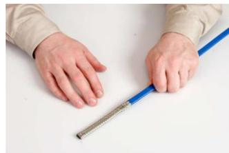
4. Push ground braid back towards the outer jacket cut back. Make a buckle in the braid. With a screw driver, create an opening in the ground braid without cutting it, big enough to pull the cable through. Bend cable enabling it to push through the opening in the ground braid. Twist the ground braid into a solid ground lead.
