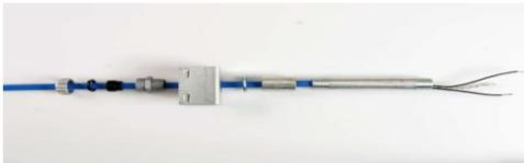
2. Disassemble the Strain Relief assembly, cut heaters on approximately a 45° angle. Lubricate heaters with cable lubricant and thread heaters through Strain Relief cap, washer and grommet respectively (wide end towards washer) until 8" (20 cm) of the heater end is exposed. Put Strain Relief base aside.
