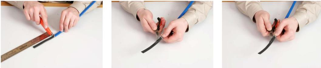
6. Notch core. Peel one of the conductors from the core. Score core between the conductors as close as possible to cut back end. Peel core from remaining conductor. Clean conductor wires until wires are completely exposed.
