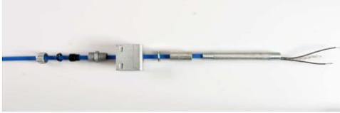
9. Feed the Heater Conductors and Ground Wire through the Strain Relief Housing up the 3" (76 mm) Nipple and into the Junction Box. Fit the Heater Strain Relief Grommet into the Strain Relief Housing. Locate the Strain Relief Nut and Washer and tighten hand tight.
