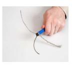
7. Place the supplied tube over one bus wire prior to sliding the core sealer over the bus wires (PGW, MT, HT only this will provide added protection from a short between the two bus wires). Then slide the core sealer over the bus wires of the cable, over the inner core until as close to the braid as possible.
