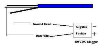
A record should be kept of the reading after the cable has been installed. This reading can be used as a reference point when taking future readings during regular maintenance.
