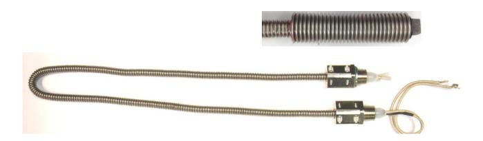
PipeGuard CMH is available from the factory as a Pre-Assembled Unit (PAU). Each PAU comes complete with a power termination at one end, a heated section in the middle and a choice of end seals for the other end. One style of end seal can either be terminated in its own junction box or be doubled back into the power junction box. The other style of end seal is low-profile and does not require any further protection.
