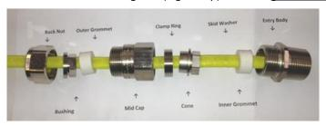
2. Disassemble the Cable Gland and install the Entry Body into the enclosure. Thread the heater through the components (less Entry Body) until the heater end is exposed.
