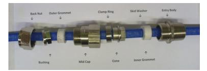
2. Disassemble the Cable Gland and install the Entry Body into the enclosure. Thread the heater through the components (less Entry Body) until the heater end is exposed.
