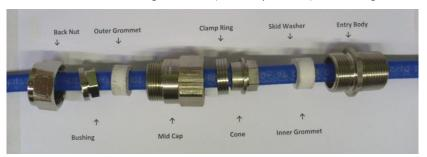
2. Disassemble the Cable Gland and install the Entry Body into the enclosure. Thread the heater through the components (less Entry Body) until the heater end is exposed
