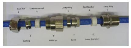
2. Disassemble each Cable Gland and install the Entry Body into the enclosure. Thread the heater through the components (less Entry Body) until the heater end is exposed
